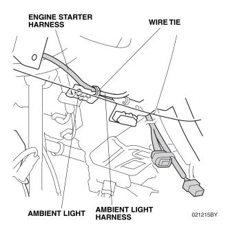
46. Using isopropyl alcohol on a shop towel, thoroughly clean the left knee bolster where the aluminum tape will attach. Attach the engine starter harness to the inside of the left knee bolster with the aluminum tape.
