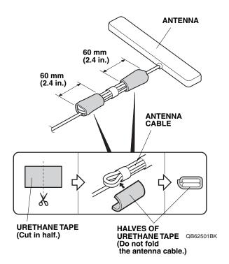
51. Using scissors, cut two urethane tapes in half. Wrap four halves of urethane tape around the antenna cable at the measurements shown.
