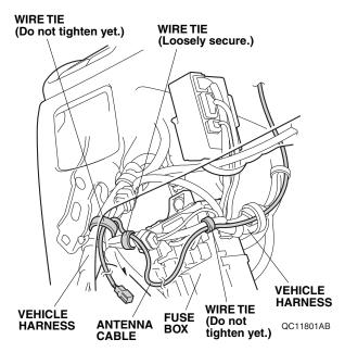
59. Loosely secure the antenna cable to the engine starter harness with one wire tie.
