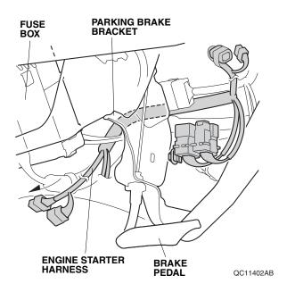
19. Secure the clip from the engine starter harness relay block to the hole in the parking brake bracket.
