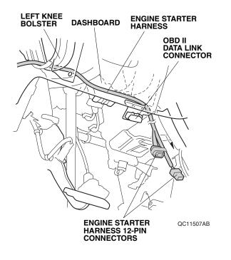
43. Align the white tape on the engine starter harness with the hole on the vehicle bracket, and secure the engine starter harness to the vehicle bracket with one wire tie.
