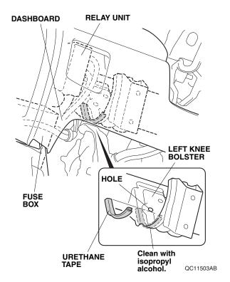
38. Unplug the vehicle 2-pin connector from the relay unit, and plug it into the engine starter harness 2-pin connector. Plug the remaining engine starter harness 2-pin connector into the relay unit.
