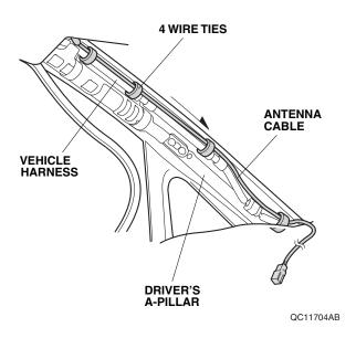
55. Route the antenna cable down and under the dashboard as shown.
