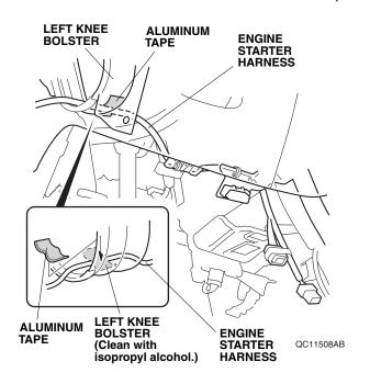
47. Continue routing the engine starter harness as shown.
