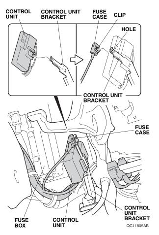
66. Attach the clip on the engine starter harness fuse case to the hole in the control unit bracket.
