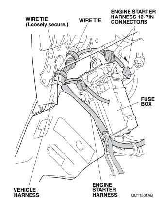
35. Secure the engine starter harness to the vehicle harness with one wire tie.
