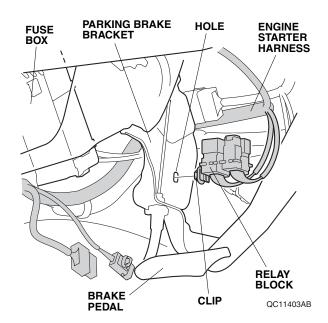
20. Secure the engine starter harness to the vehicle harness with one wire tie.
