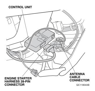
65. Install the control unit to the control unit bracket.
