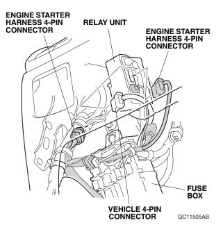
40. Locate the 4-pin connector taped to the vehicle harness, and remove the tape to release the connector. Plug the engine starter harness 4-pin connector into the vehicle 4-pin connector.
