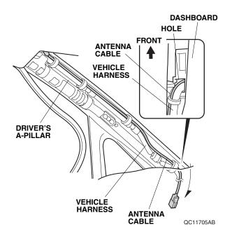
56. Route the antenna cable along the vehicle harness, and secure it to the vehicle harness with one wire tie.
