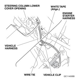
22. Align the white tape on the engine starter harness with the vehicle clip, and secure the engine starter harness to the vehicle harness with one wire tie as shown.
