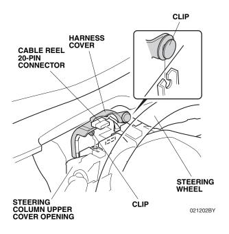
27. Route the engine starter harness through the steering column area as shown.
