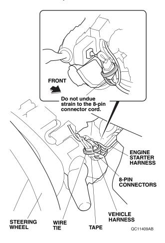
32. Secure the engine starter harness to the vehicle harness with one wire tie.
