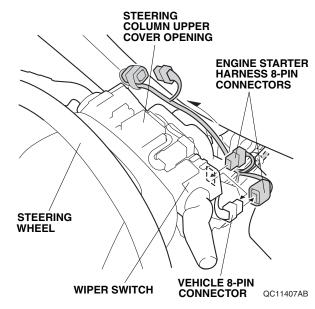
25. Unplug the vehicle 8-pin connector from the wiper switch, and plug it into the engine starter harness 8-pin connector. Plug the remaining engine starter harness 8-pin connector into the wiper switch.
