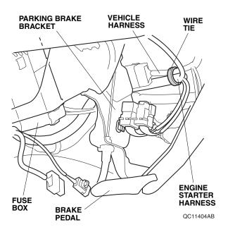
21. Align the white tape on the engine starter harness with the vehicle clip, and secure the engine starter harness to the vehicle harness with one wire tie.
