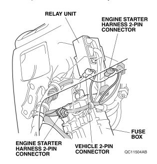
39. Unplug the vehicle 4-pin connector from the relay unit, and plug it into the engine starter harness 4-pin connector. Plug the remaining engine starter harness 4-pin connector into the relay unit.
