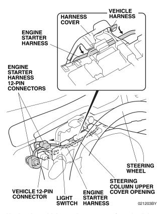
28. Unplug the vehicle 12-pin connector from the light switch, and plug it into the engine starter harness 12-pin connector. Plug the remaining engine starter harness 12-pin connector into the light switch. 29. Secure the 12-pin connectors and the engine starter harness with one wire tie.
